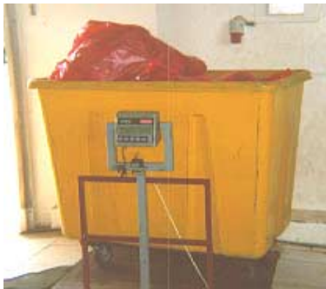
Photo 5. Four-wheeled trolley for transporting sealed waste bags: the top cover is open
