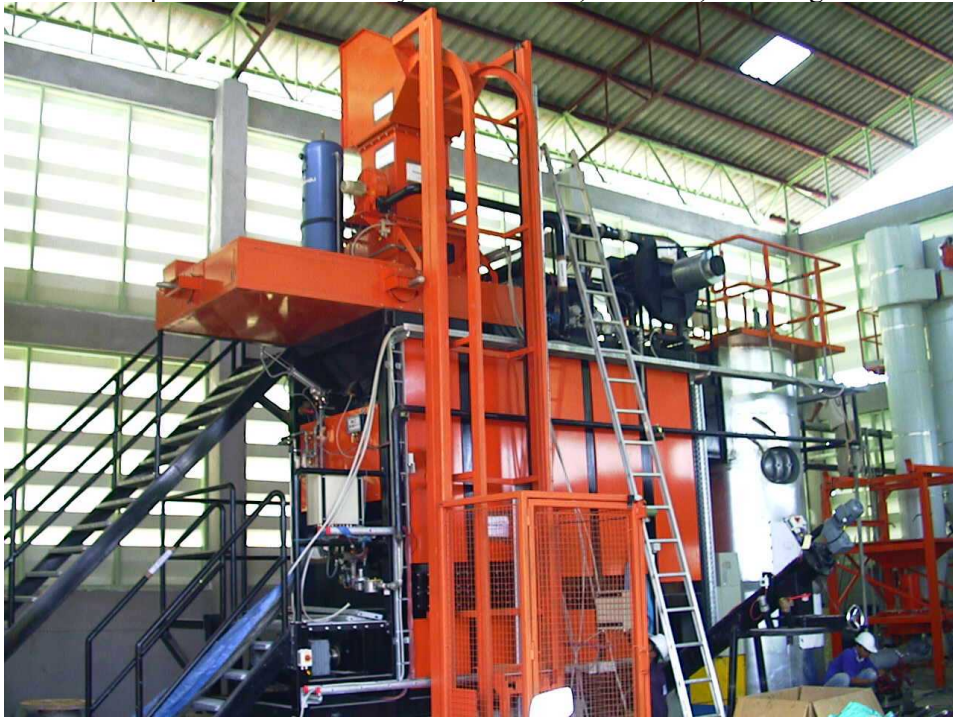
Figure 6.4: Example of a dual chamber incineration plant for health care risk waste with flue gas cleaning
