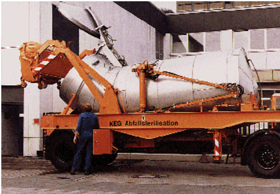
Box 6.5 B: Example of a mobile steam sterilisation plant (autoclave plant)
