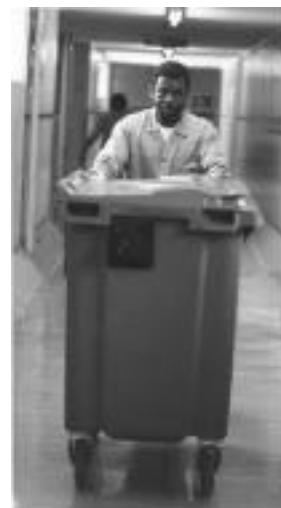
Red wheelie bins are used for the internal transportation of health care risk waste
